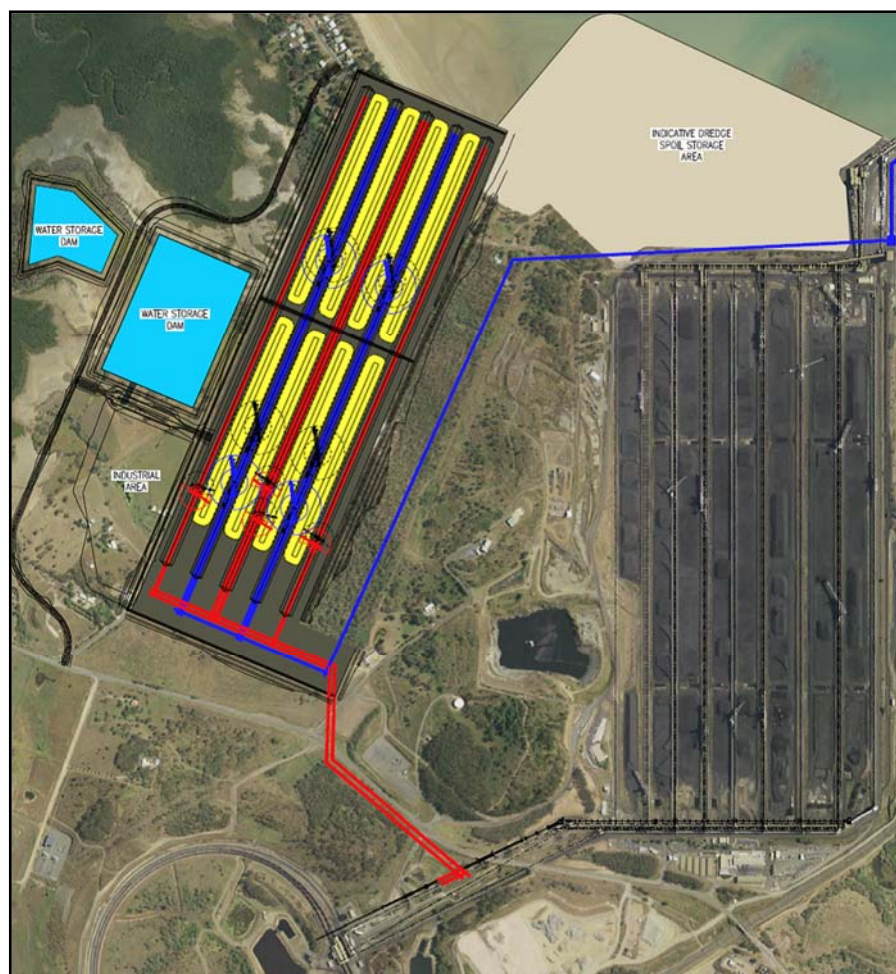
Figure 40: 'Long' stockyard arrangement suited to configuration options 2 and 3.
