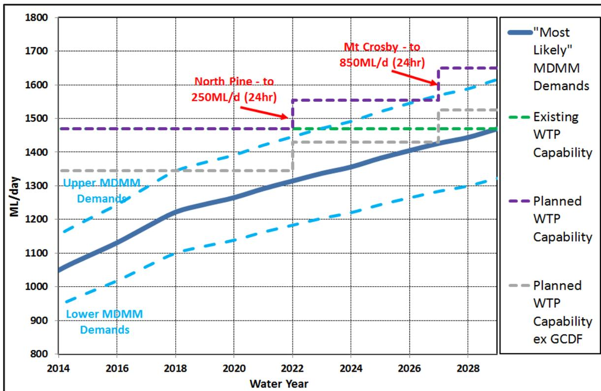
**Figure 8: Connected Bulk Water Supply System MDMM Demands and WTP Capability**
