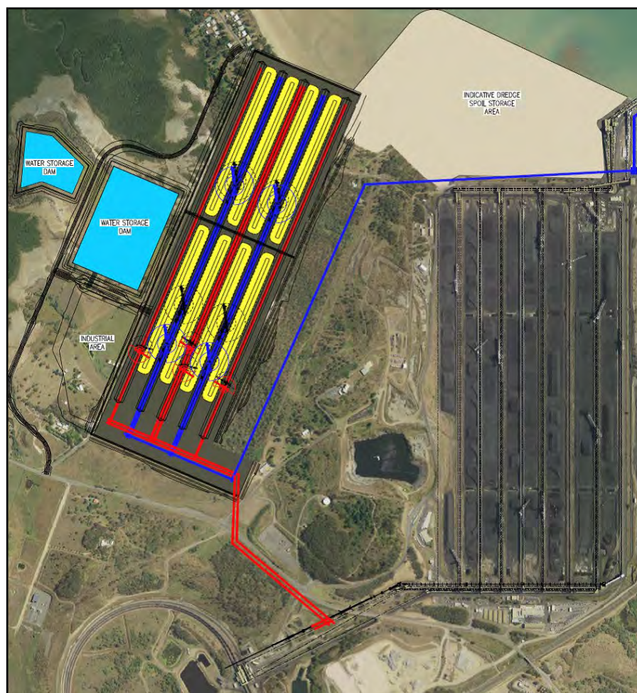
Figure 41: 'Long' stockyard arrangement suited to configuration options 2 and 3.
