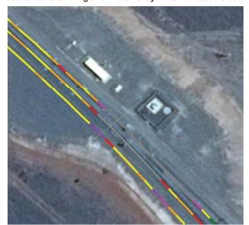
Figure 24.1 - GPR Results at Caval Ridge Turnout. Grey lines indicate no data available
