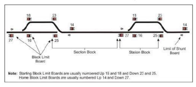
Figure 8: DTC Blocks and Position of Block Limit Boards
