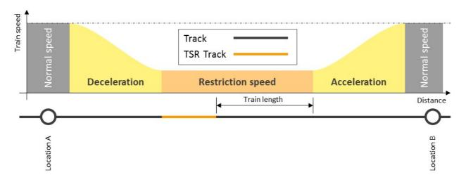
Figure 14: Assumed impact to train speed used to calculate TSR impact to SRT
