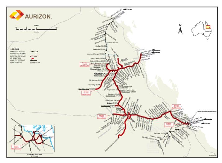
Figure 9: Electrification of CQCN.
