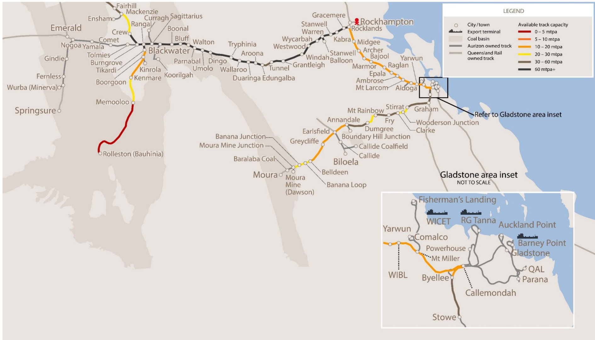
Figure 18: Heat map of Blackwater and Moura System branch line capacity
