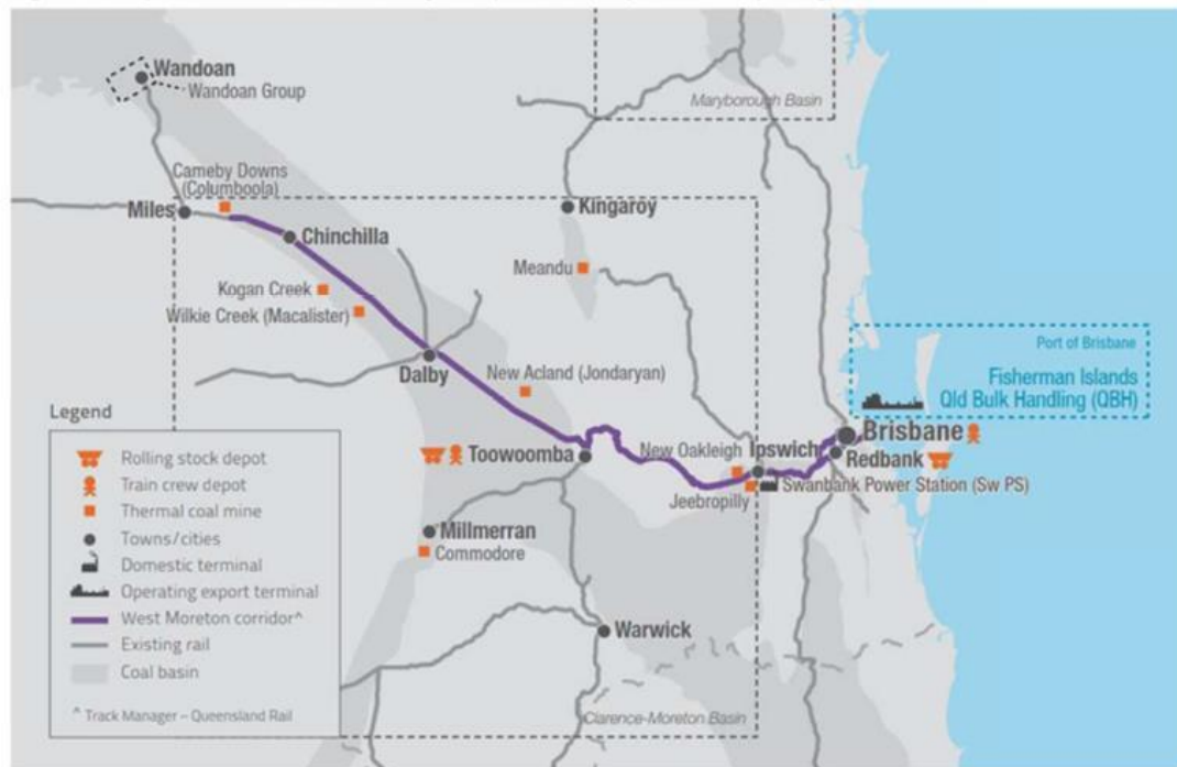
Figure 13 The West Moreton corridor rail transport infrastructure
