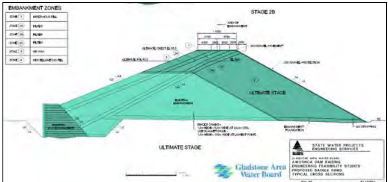
Figure 9-1 Awoonga Dam Feasibility Study Proposed Saddle dam Typical Sections
