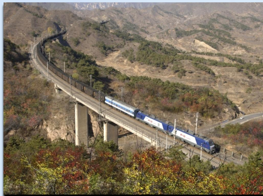
HX d 2机车大秦线上牵引两万吨煤炭 HX d 2 locomotive 20,000t heavy haul coal freight for China Da-Qin railway
