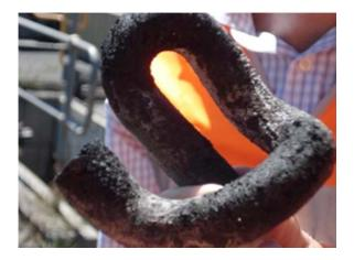
Figure 6: Coal Corroded Fishplate
