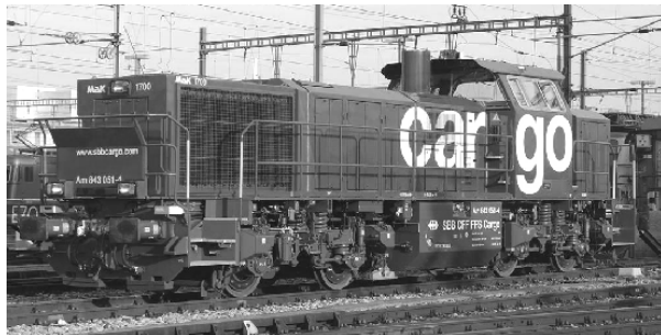
Particles are burned in a SiC filter Diesel engine: CAT 3512
