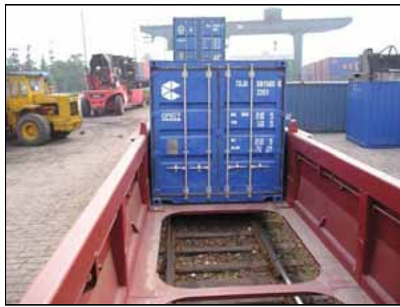
Photo 5-2 The Internal Structure of the Well-type Wagon (Shanghai)
