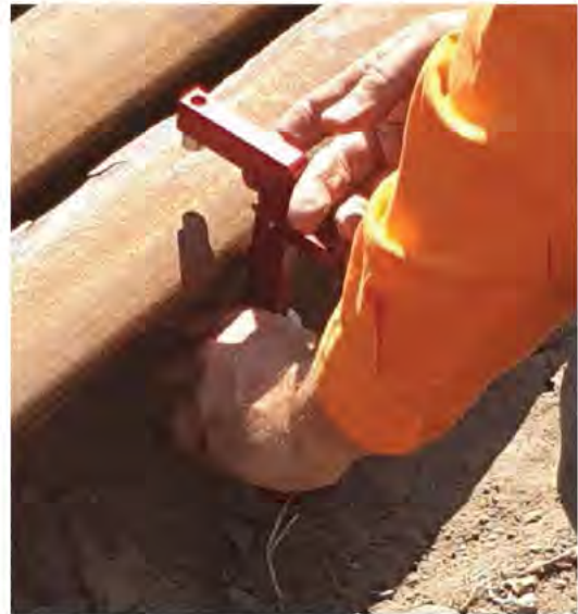
Figure 7.6 – Field table wear measurement on removed rail
