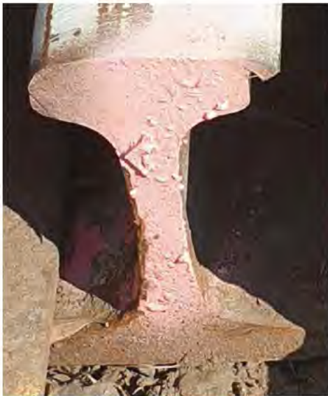
Figure 7.5: Head flow and table wear on removed rail 30
