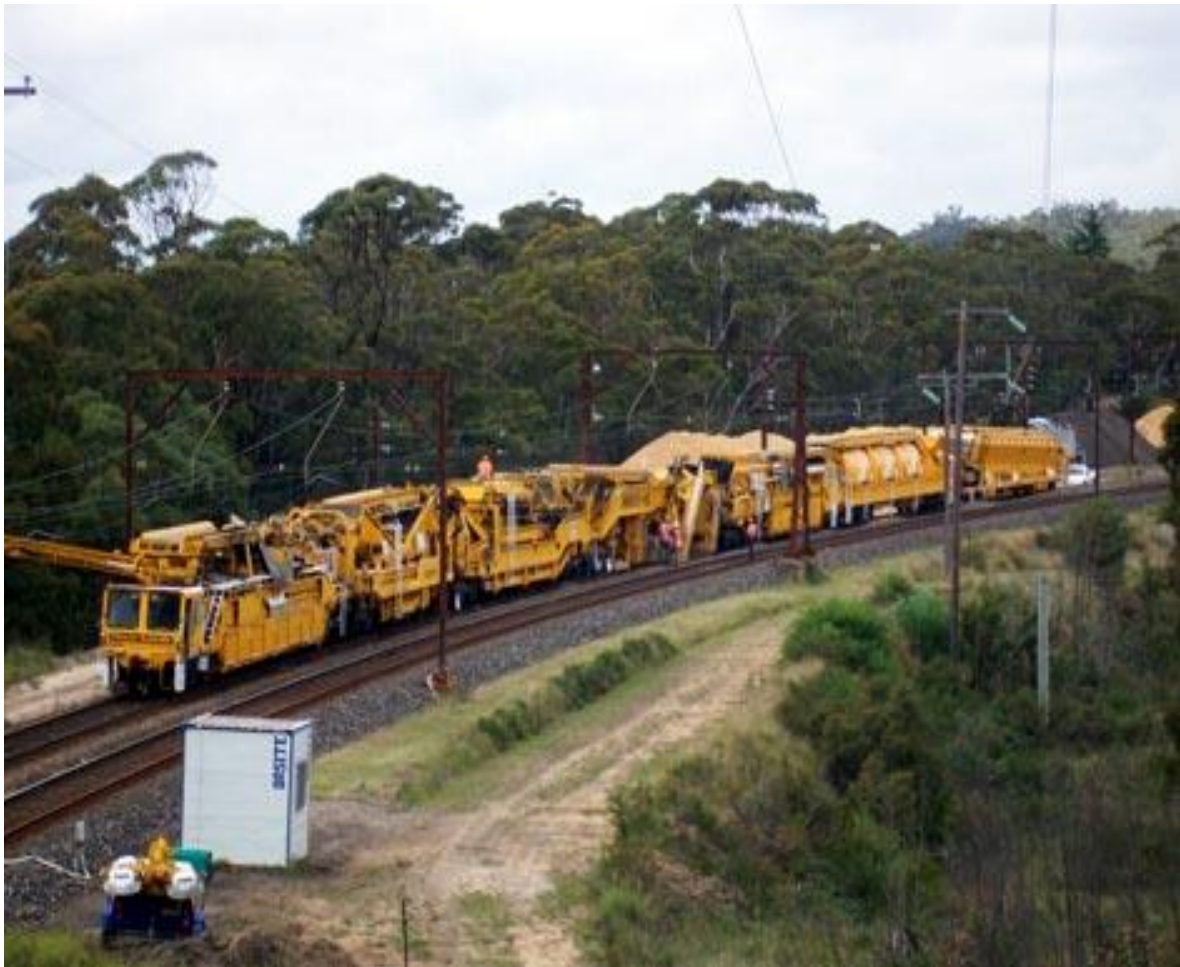
Figure 2 RM-900 mainline ballast undercutting machine
