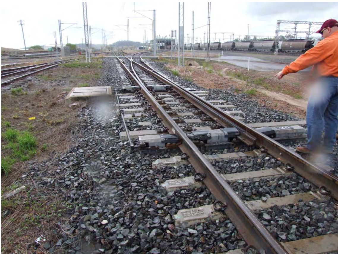
Figure 8: Siemens switch motor fitted with switch rollers
